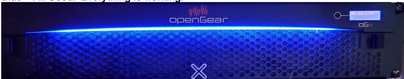
Figure 5-1. Blue Indicates the System is Fully Functional with no Alarms
