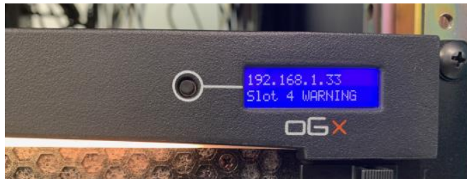
Figure 1-13. LCD Display on the openGear Frame's Front Panel
